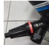
Assemble and connect the Pressure Relief Valve, ensure that the Valve's exhaust is horizontal.
